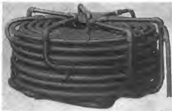
White Generator, Showing Coil Connections.
